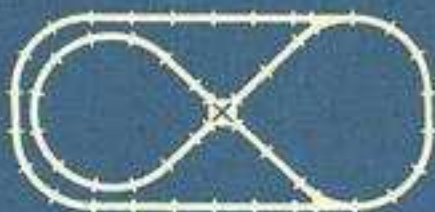
No. 3—Space 32" x 100" Track: 21 Curve, 18 Straight, 4— \frac{1}{2} Straight, 2— \frac{1}{2} Curve, 1 pair Switches, 1 Crossover
