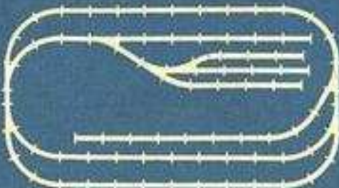
No. 30—Space 65" x 120" Track: 22 Curve, 32 Straight, 4 Right Switches, 3 Left Switches, 2— \frac{1}{2} Straight
