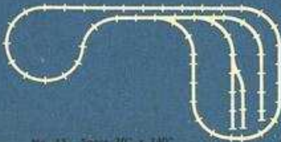
No. 13—Space 70" x 140" Track: 28 Curve, 26 Straight, 4— \frac{1}{2} Straight, 2 Right Switches, 1 Left Switch
