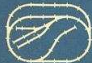
No. 26—Space 50" x 70" Track: 19 Curve, 14 Straight, 1— \frac{1}{2} Straight, 4 Left Switches, 2 Right Switches
