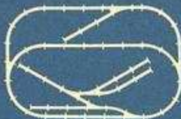
No. 11—Space 60" x 90" Track: 26 Straight, 16 Curve, 4— \frac{1}{2} Straight, 3 Left Switches, 3 Right Switches
