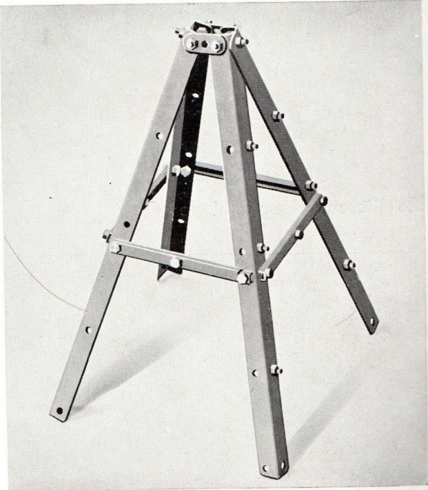
1.12 Signal de triangulation
