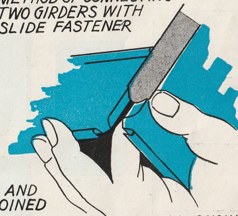
METHOD SHOWING CONNECTION OF TWO PANELS WITH SLIDE FASTENER
