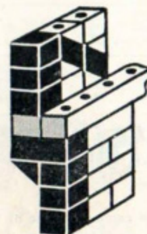
Fig. 10—Showing a method of constructing overhanging storey.
