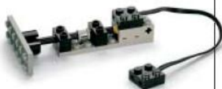
A bumper that uses one touch sensor
