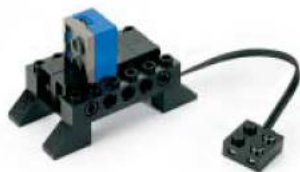
A bumper that uses two touch sensors
