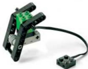
A bumper that uses one touch sensor
