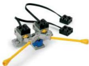
A bumper that uses two touch sensors
