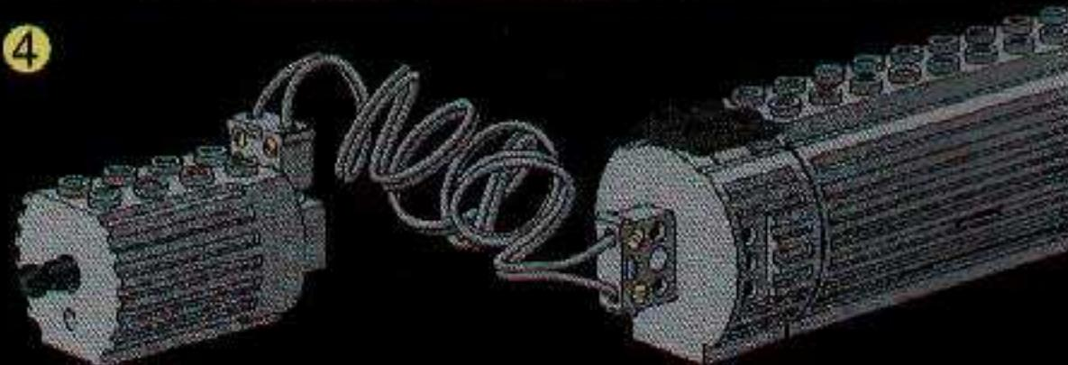
The motor and battery rod are connected with a wire. When the switch is in the centre position, the current is cut off. In the outer positions the motor goes forwards or backwards. If the switch is only pressed lightly, it will automatically return to the centre position when you let go.
