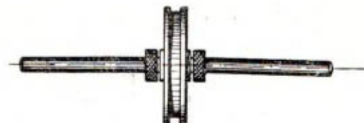
Showing a revolving wheel fixed between 2 Spring Washers on a Standard Bar.
