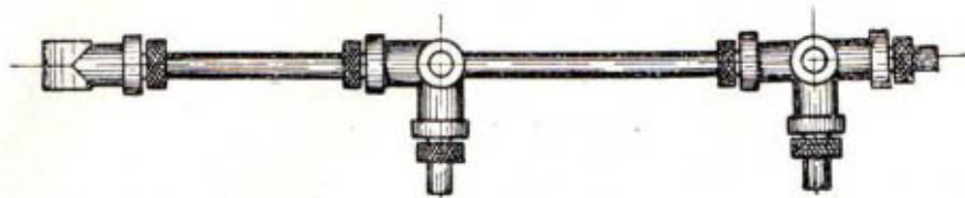
Showing the principal joints fixed to a Standard Bar by means of Spring Washers.
