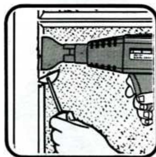
The nozzle has been designed to deflect heat away from glass or other fragile areas onto the work surface.
